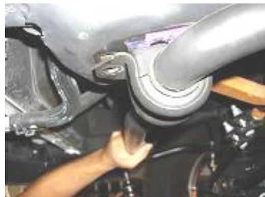
4. Snug torsion sway bar brackets to the frame with factory or supplied hardware. The Bushing lip will be on the outside of the bracket (facing the tire) and the bushing should be offset forward (The passenger side is pictured). Apply a small amount of grease inside the bushing for easier install of the torsion bar.
