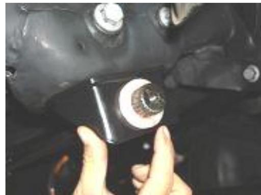
7. Insert supplied pinch bolt into the end of one of the arms with the nut side down, do not tighten. Push the arm onto the splines of the torsion bar and secure using supplied  $5/16$ -24 X 1" bolt, lock washer, fender washer. Install Arm on other side and insert  $5/16$ "x1" on the bar. Snug by hand to ensure even spline engagement. Once even, torque both  $5/16$ " bolts to 33 ft. lbs.
