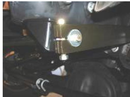
9. Thread the heim joints away from the jam nuts and apply loctite to the threads where the jam nuts will be torqued.
