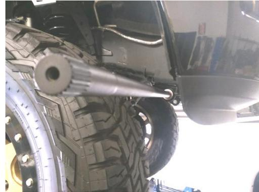
6. Tap torsion bar through until it is centered. There should be  $\frac{3}{4}$ " of the bar sticking out from the end of each bushing. Once aligned, Torque Sway bar drop bracket hardware to 35ft. lbs.
