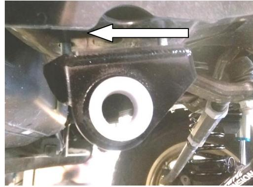
5. Align torsion bar with driver side bushing and tap it through to the passenger side using a rubber mallet.
